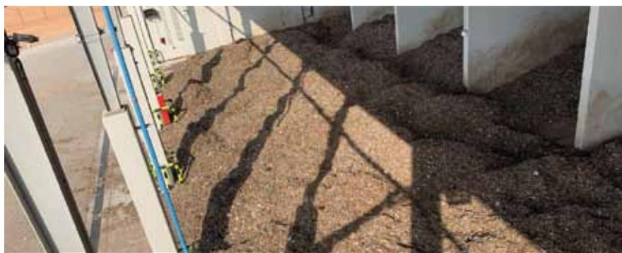
The particle size of the fuel must be small enough to allow rapid and complete combustion in the calciner and allow as many cement plants as possible to use the alternative fuel without major modifications
