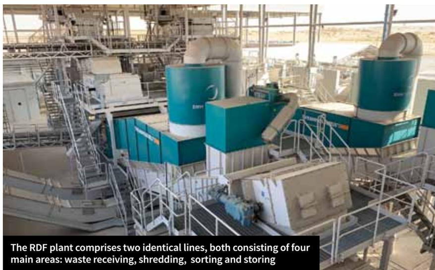
The RDF plant comprises two identical lines, both consisting of four main areas: waste receiving, shredding, sorting and storing
